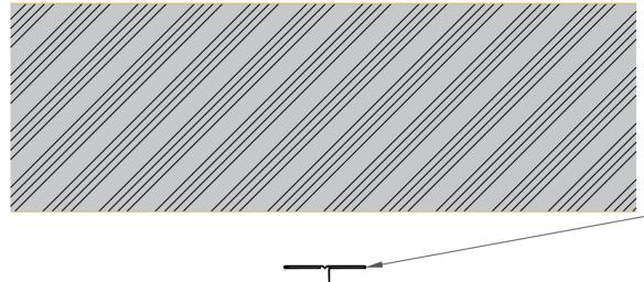
SPEEDLINE 50mm 'I' Studs at 600mm Ctrs
