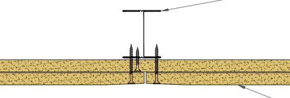
2x12.5mm Siniat GTEC Standard Board fixed with SPEEDLINE Drywall Screws at 300mm centres (200mm centres at external angles). Ref to table for fixing length.
